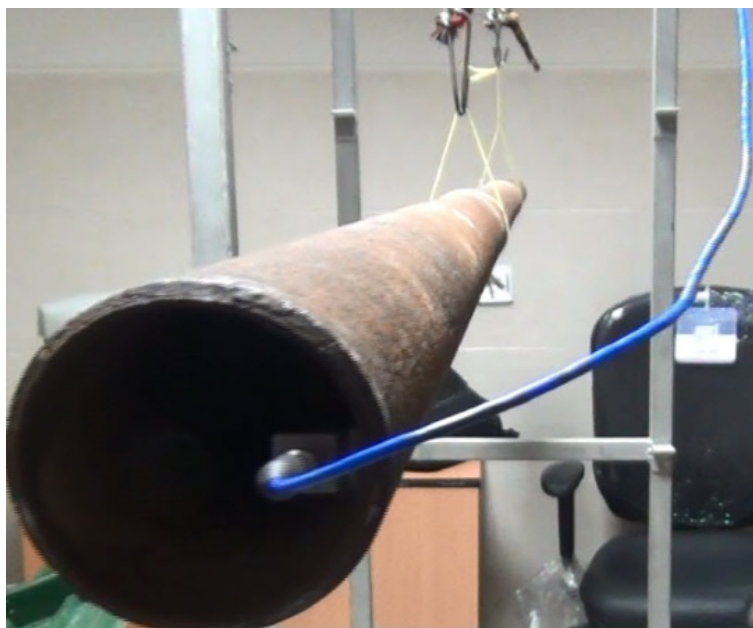
Figure 3. Modal Analysis of the sample pipe
